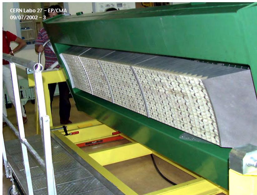
Figure 4.2: Photograph of supermodule, showing modules.
