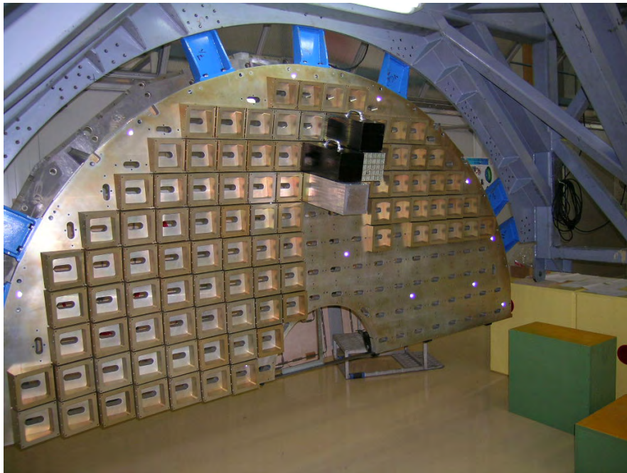
Figure CP 8: The 60 mm thick aluminium backplate of an ECAL endcap Dee held on its assembly and installation frame. Four mock supercrystals ( 5 \times 5 crystals) are shown attached in position along with all 138 positional spacers.
